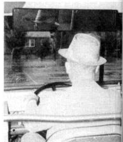
THE SMALLER overhead rear-view mirror in the picture at left is being replaced by the large one at right. This increases the school bus driver's scope of vision by many times.
