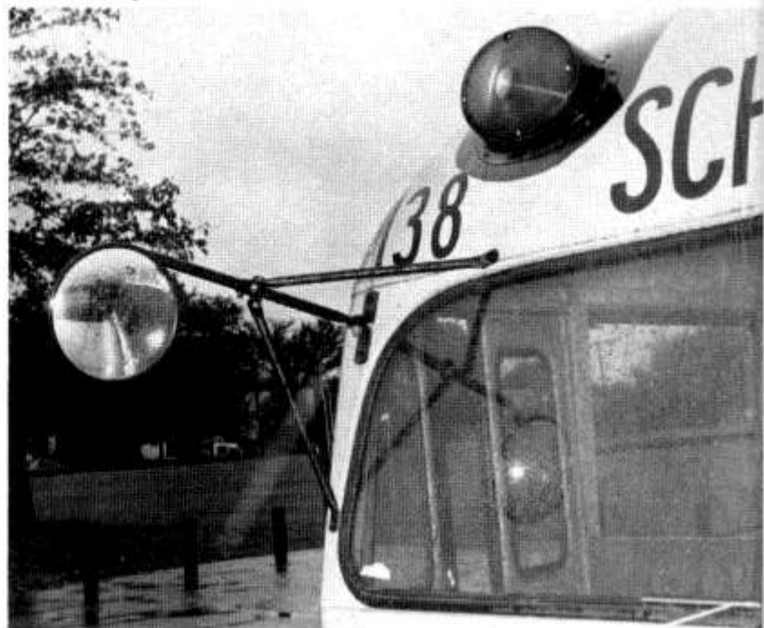
THIS CROSS-VIEW mirror enables the driver to see the ground directly in front of the hood of his school bus. It is an important safety advance, since otherwise it would be possible for a small elementary-aged child to "disappear" in front of the hood.
