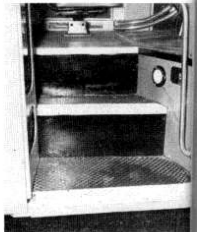
THE METAL step tread at left is being replaced by an improved rubber tread shown at right. The new non-skid tread permits faster drainage of water from the step and provides a sure footing for students.
