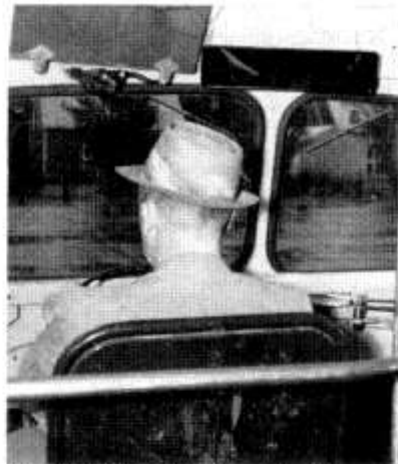
THE SMALLER overhead rear-view mirror in the picture at left is being replaced by the large one at right. This increases the school bus driver's scope of vision by many times.
